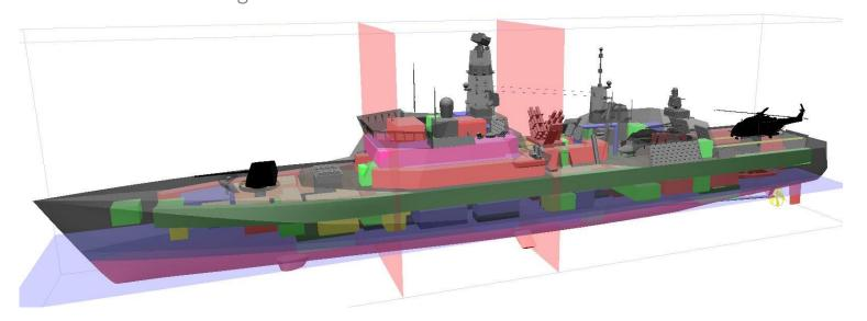
Blastproof doors are provided, whilst blastproof bulkheads are optional. System positioning has been used to reduce vulnerability whilst allowing for a reduction in capability for design to cost.
